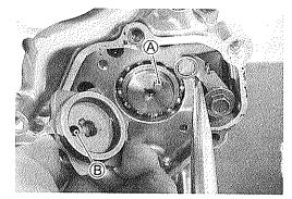
Apply a small quantity of THREAD LOCK "1342" to the gearshift cam stopper plate bolt ① and tighten it to the specified torque.
