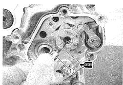
Assembly the geafshift shaft/gearshift arm.
