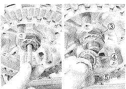
• Tighten the clutch spring set bolts diagonally to the specified torque while holding the generator rotor with the special tool.
