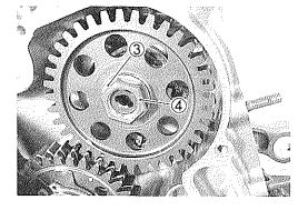
• Hold the generator rotor with the special tool.
