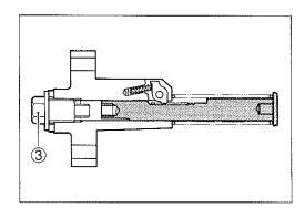
$\bullet$  Compress the cam chain tension adjuster rod 1 fully by releasing the ratchet 2.
