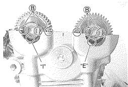
· Install the dowel pins.
