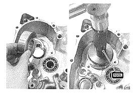
• Install the bearing retainers.
