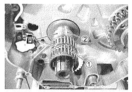
• Install the primary driven gear assembly 1 onto the countershaft.
