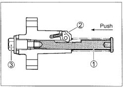
• From this position, turn out the cam chain tension adjuster bolt ③ until locking the cam chain tension adjuster rod ①. Now the cam chain tension adjuster is ready to install.
