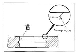
• Set the bearings installed in the special tool to the crankcase half as shown.
