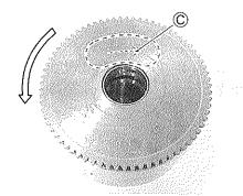
Inspect the starter driven gear bushing for any damage.
