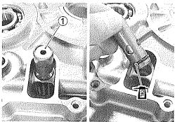
Check the operation of the oil pressure regulator by pushing on the piston with a proper bar. If the piston does not operate, replace the oil pressure regulator with a new one.
