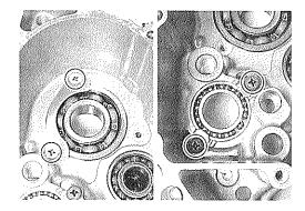
• Remove the bearings with the special tool.
