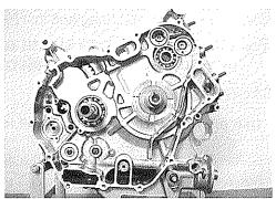
• Install the engine sprocket spacer ① onto the driveshaft.
