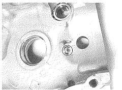
Check the oil jets for clogging. If they are clogged, clean their oil passage with a proper wire or compressed air.
