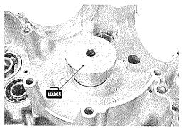
Gradually press out the bearing with the special tool by using the hand-press.
