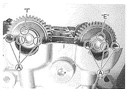
Install the dowel pins.
