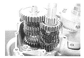
Install the gearshift forks and gearshift cam.
