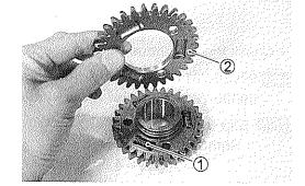
• Install the spring washer 3 not to cover the holes of the gears.
