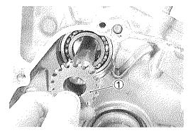
Degrease the tapered portion of the generator rotor assembly and also the crankshaft. Use nonflammable cleaning solvent to wipe off oily or greasy matter and make these surfaces completely dry.
