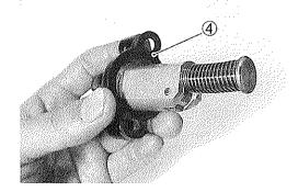
Install the cam chain tension adjuster as shown and tighten its mounting bolts to the specified torque.
