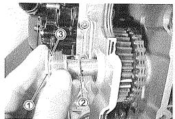
• Check and correct the positions of the "F I T" line on the generator rotor and cam drive idle gear/sprocket ①.
