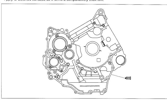
When securing the right and left crankcase halves, tighten each bolt a little at a time to equalize the pressure. Tighten all the securing bolts to the specified torque values.
