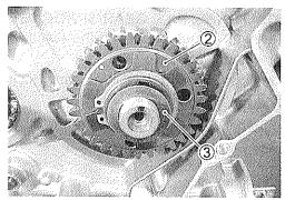
• Install the primary drive gear nut.
