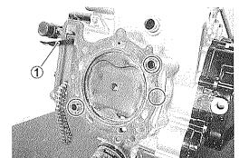
• Place the rear cylinder head on the cylinder.
