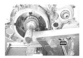
• While holding the generator rotor, tighten the cam drive idle gear/sprocket nut to the specified torque.
