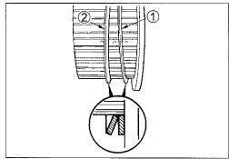
Insert the clutch drive plates and driven plates one by one into the clutch sleeve hub in the prescribed order, No.3 drive plate being inserted first.
