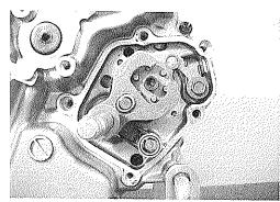
• Install the dowel pins and gasket ②.
