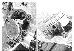
Apply engine oil to the sliding surface of the pistons and cylinders.
