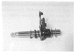
Install the gearshift shaft as shown.
