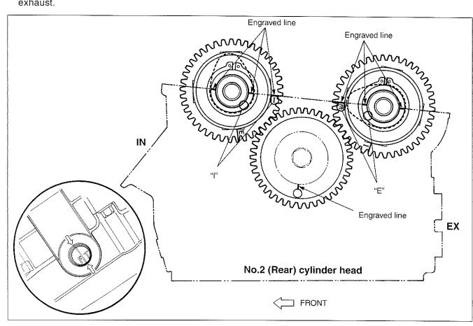
After installing the No.2 (Rear) camshafts, rotate the generator rotor 360 degrees (1 turn), and recheck the positions of the camshafts.
