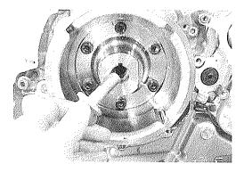
• While holding the generator rotor with the special tool, tighten the bolt to the specified torque.
