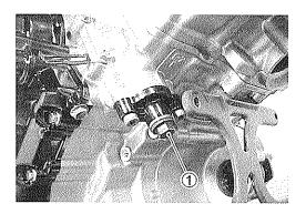
• Tighten the cam chain tension adjuster bolt ① to the specified torque.
