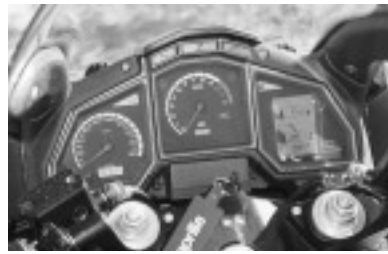
Above: Two analog gauges; the speedo and tach, are included in a multifunction digital panel featuring a clock, ambient air temp, water temp, liters of fuel remaining (displayed graphically and numerically) and "service" messages including any fuel injection malfunction. The lighting is blue on black—very trick.
