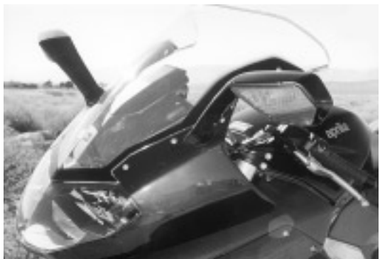
Below: Pointy nose and triple headlight arrangement make the Futura's styling unique. The faceted, angular bodywork is very good at evading radar, too! The mirrors, with the turnsignals built into their forward edges, remind us of the invaders from H.G. Wells' War of the Worlds . Unfortunately, they vibrate on their stalks and are too far from the rider to do an adequate job of revealing traffic. However, they do make the front turnsignals easy to see.
