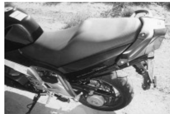
Below: Futura's seating is well-shaped and comfortable for the long haul. The rear spring preload can be adjusted on the fly (carefully) by a knob just under the edge of the rider's thigh. Single-sided swingarm makes tire changes and chain adjustment a snap and a centerstand is also standard. Rectangular openings beneath the rear bodywork and small bracket attached to the passenger peg bracket support the saddlebags.
